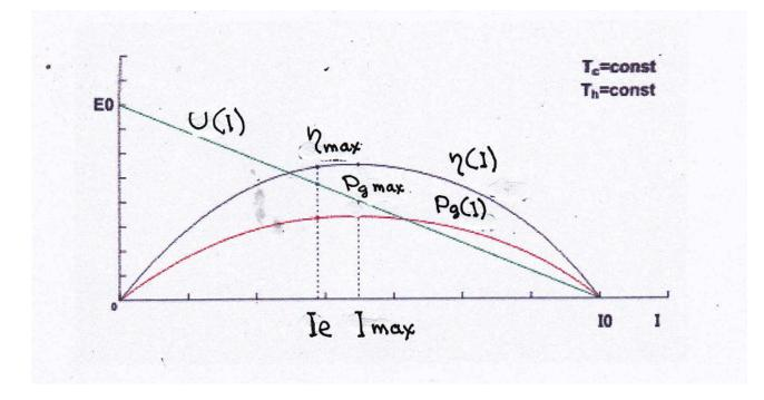
Formulae describing the device: thermoelectric generator
