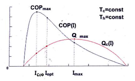
The temperature difference that occurs in the module is determined not only by the processes inside the thermocouple, but also by the magnitude of the thermal load on the cold surface of the module. The less heat flow from the environment onto a cold surface, the more its temperature can be reduced.
